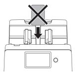
When scanning cards, clear the [Detect by Ultrasonic] check box in the [Error Detection] tab on the scanner driver settings screen. (See p. 31)
