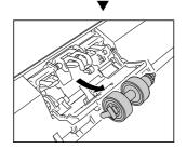
Install the new retard roller by inserting the right side first.
