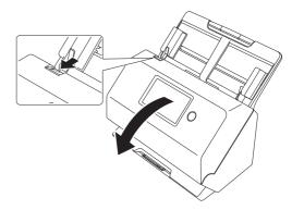
Use compressed air to remove dust and paper particles from the inside of the scanner.
