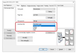
If [Skip Blank Page] is selected, the [Setting] button is enabled, and you can adjust the level for judging whether pages are blank.
