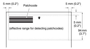
Keep the patchcode sheet clean. Take particular care to keep the patchcode detection range area clean. Also, do not bend, fold or crease the sheet.
