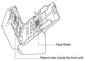
When closing the front unit, make sure that it is completely closed by gently pressing the left and right until you hear a click.
