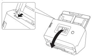
Use compressed air to remove dust and paper particles from the inside of the scanner.
