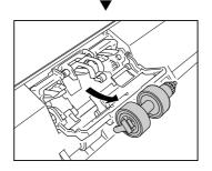
Check that part A is up and first mount the right side of the new retard roller to the scanner from under part A.
