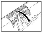
Pull the left lever that secures the retard roller to the scanner, and remove the roller.
